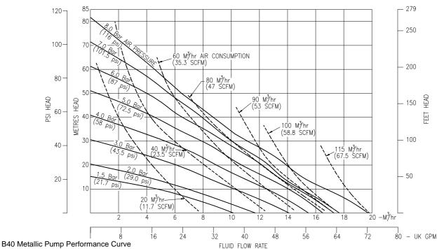
Performance based on water at ambient temperature
